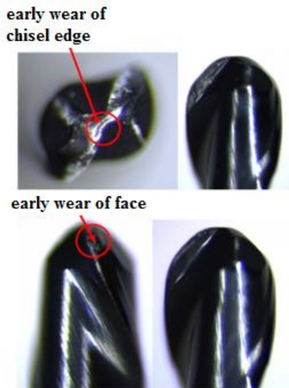
Fig. 7. Tool wear at 40% of the tool life
