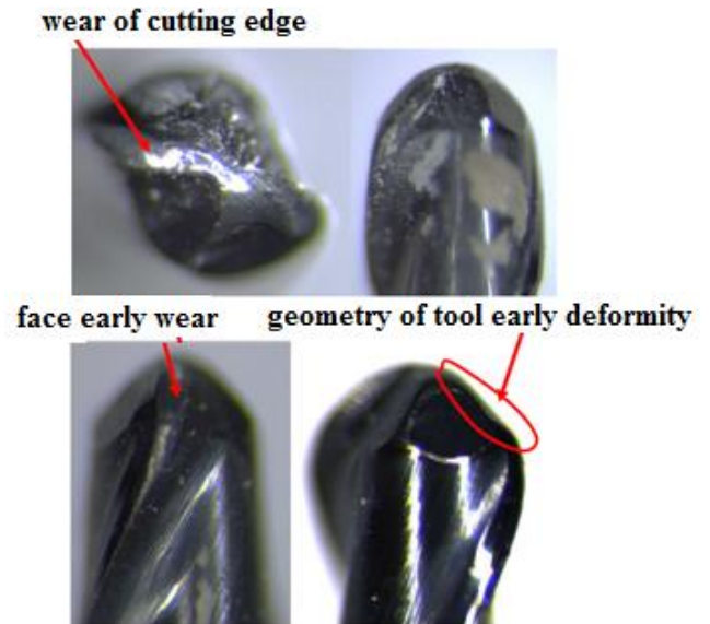
Fig. 8. Tool wear at 60% of the tool life
