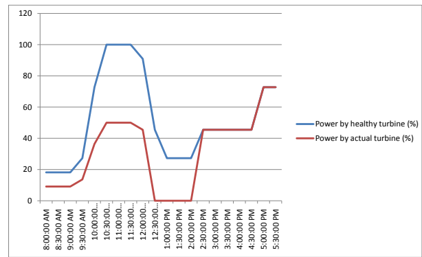
Fig. 2. General degradation. The upper (blue) line corresponds to the expected production of a healthy turbine over time, given the forecasted wind speed. The lower (red) line shows the expected production given the current failure and the maintenance schedule. Production is degraded by 50% until 10:00, when the turbine is stopped for maintenance, at the end of which it is restored into a healthy state.
