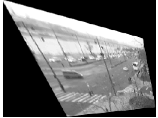
Fig. 7. Image (a) is the view seen by the left-hand camera; (b) is the transformed view seen by the right-hand camera, without “fine-tuning”. The matching is poor: edges that are continuous appear broken if a composite view is generated from the two images.
