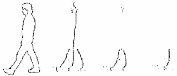
Figure 1. An idealised outline of a walking person, together with the derived Level 1, Level 2, and Level 3 symmetry maps.
