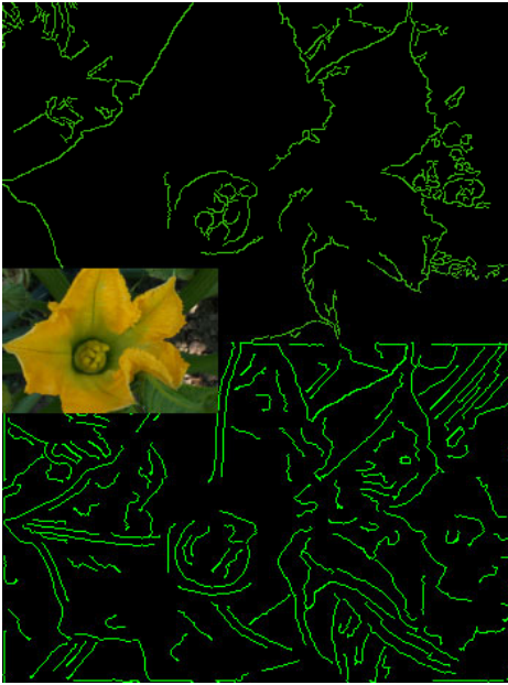
Figure 3: Example of Canny (3x3, hysteresis parameters 30 and 200, up) and multiscale-detected edges which is used for painting (down).
