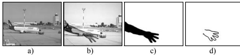
Fig. 2. Steps of the contour segmentation; a) Input image; b) camera image with arm; c) segmented arm image; d) extracted palm contour
