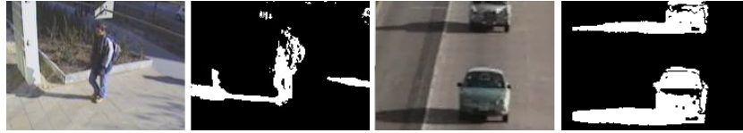
Fig. 1. Results of foreground detection with Stauffer-Grimson algorithm. Left: School Entrance in the afternoon ('SE pm') video, right: 'Highway' test sequence.
