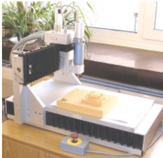
Figure 5. The 3D milling machine controlled by the prototype CNC
