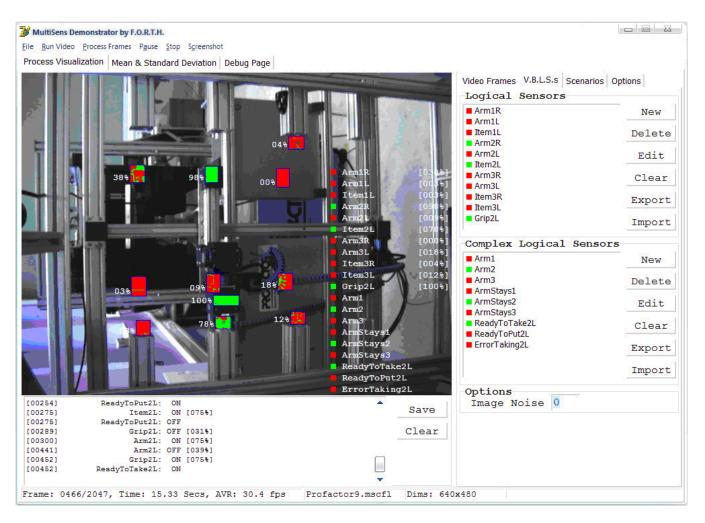
Figure 5: Graphical user interface of the prototype program; the rectangles on the video represent regions of interest, their colors (green/light – red/dark) indicate the output of the appropriate visual sensor at the current frame
