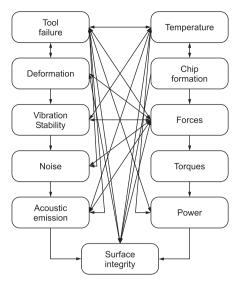
Fig. 1. A practical example for complexity: key interdependencies for a cutting process (Peklenik and Jerele, 1992). Each basic node may contain numerous parameters—the total number of variables can easily go into the hundreds for such industrial processes.
