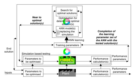
Fig. 3. Concept of the hybrid, AI-, ML- and simulation-supported optimisation of production plants
