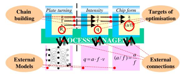
**Fig. 1.** Hybrid modelling and optimisation by ProcessManager (model of the plate turning operation with optimisation criteria)
